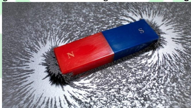
Iron filings near the bar magnet align themselves along the field lines
