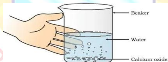
Formation of slaked lime by the reaction of calcium oxide with water
