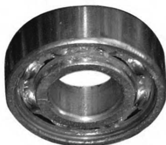
Fig. 12.16 : Ball bearings reduce friction
