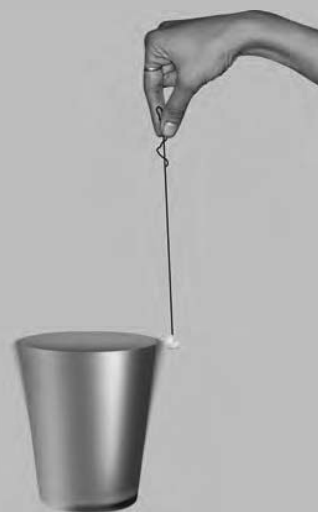
Fig. 13.17 : Thermocole ball touching the vibrating glass tumbler
