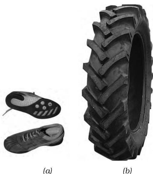
Fig. 12.11 : Soles of shoes and tyres are treaded to increase friction
