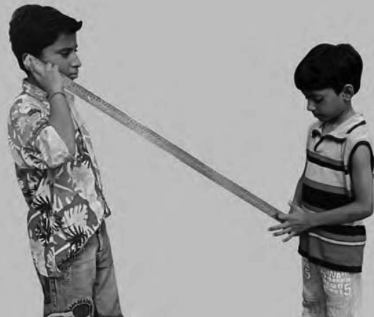
Fig. 13.12 : Sound travelling through a metre scale
