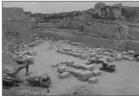
Fig. 3.7: Quarrying of limestone
